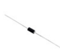
P6KE13A Littelfuse Inc. TVS DIODE 11.1VWM 18.2VC DO204AC
