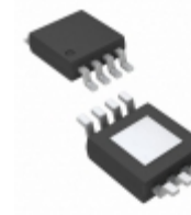
RT9069-33GSP Richtek USA Inc. IC REG LDO 3.3V 0.2A 8SOP
