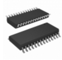
AD876JR Analog Devices Inc. IC ADC 10BIT 20MSPS CMOS 28-SOIC
