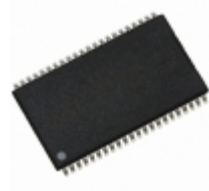
IS62WV25616DALL-55TI -TR ISSI, Integrated Silicon Solution Inc IC SRAM 4MBIT 55NS 44TSOP
