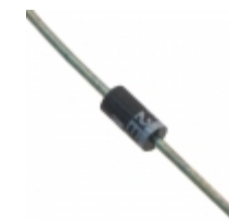
1N4742A G Microsemi Corporation DIODE ZENER 12V 1W DO204AL
