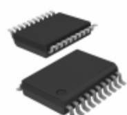
PIC16C54T-RC/SS Microchip Technology IC MCU 8BIT 768B OTP 20SSOP
