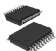
PIC16C54T-RCE/SS Microchip Technology IC MCU 8BIT 768B OTP 20SSOP
