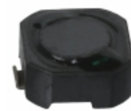
CDRH62BNP-150MC-B Sumida America Components Inc. FIXED IND 15UH 900MA 230 MOHM
