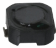
CDRH62B-680MC Sumida America Components Inc. FIXED IND 68UH 420MA 1.07 OHM
