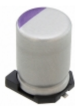
20SVPF390M Panasonic Electronic Components CAP ALUM POLY 390UF 20% 20V SMD
