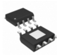
ADP7105ARDZ-5.0 Analog Devices Inc. IC REG LDO 5V 0.5A 8SOIC
