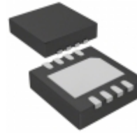
ADP7105ACPZ-1.8-R7 Analog Devices Inc. IC REG LDO 1.8V 0.5A 8LFCSP
