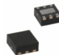
MIC5320-SOYMT-TR Microchip Technology IC REG LDO 3.3V/2.9V 0.15A 6TMLF
