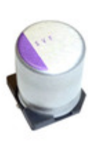
35SVF39M Panasonic CAP ALUM POLY 39UF 20% 35V SMD
