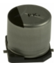
EEE-FK2A330P Panasonic Electronic Components CAP ALUM 33UF 20% 100V SMD
