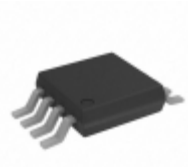
ADA4062-2ARMZ Analog Devices Inc. IC OPAMP JFET 1.4MHZ 8MSOP
