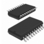
ATTINY816-SFR Microchip Technology IC MCU 8BIT 8KB FLASH 20SOIC
