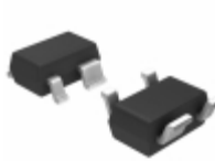
S-1000N19-N4T1G SII Semiconductor Corporation IC VOLT DETECT N-CH 19V SC-82AB
