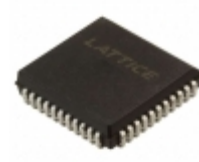
ISPLSI 2032A-150LJN44 Lattice Semiconductor Corporation IC CPLD 32MC 5.5NS 44PLCC
