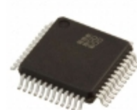
ISPLSI 2032A-180LTN48 Lattice Semiconductor Corporation IC CPLD 32MC 5NS 48TQFP
