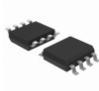
AT45DB021D-SSH-T Microchip Technology IC FLASH 2MBIT 66MHZ 8SOIC
