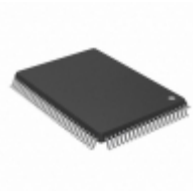
MB90F949APQC-GS-SPERE2 Cypress Semiconductor IC MCU 16BIT 256KB FLASH 100QFP
