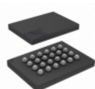
S25FL512SAGBHV13 Cypress Semiconductor IC FLASH 512M SPI 133MHZ 24BGA
