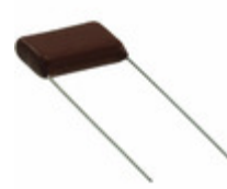
ECQ-E6104RJf Panasonic Electronic Components CAP FILM 0.1UF 5% 630VDC RADIAL
