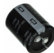
EET-UQ2W151JF Panasonic Electronic Components CAP ALUM 150UF 20% 450V SNAP
