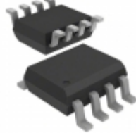
ADM1232ARNZ-REEL7 Analog Devices Inc. IC SUPERVISOR FOR CPU 8SOIC
