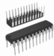
ATF20V8B-10PU Microchip Technology IC PLD 8MC 10NS 24DIP
