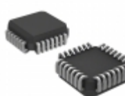
ATF20V8B-15JI Microchip Technology IC PLD 8MC 15NS 28PLCC
