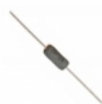
SP3AJT56R0 Stackpole Electronics Inc. RES FUSE 56 OHM 4W 5% AXIAL
