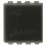
AON6538 Alpha & Omega Semiconductor Inc. MOSFET N CH 30V 30A 8DFN
