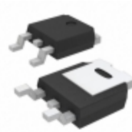
LDF33DT-TR STMicroelectronics IC REG LDO 3.3V 1A DPAK
