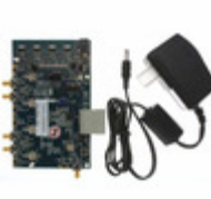
AD9259-50EBZ ADI (Analog Devices, Inc.) BOARD EVAL FOR LFCSP A/D CONV
