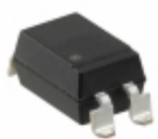
PS2501AL-1-E3-Q-A CEL OPTOISOLATOR 5KV TRANS 4SMD
