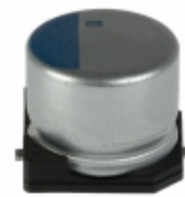
APXA200ARA470MH70G United Chemi-Con CAP ALUM POLY 47UF 20% 20V SMD
