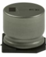
EEV-EB2D470SM Panasonic Electronic Components CAP ALUM 47UF 20% 200V SMD
