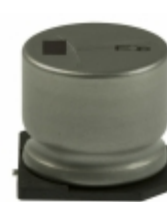
EEV-EB2E330SM Panasonic Electronic Components CAP ALUM 33UF 20% 250V SMD
