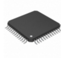
CY7C136-25NXT Cypress Semiconductor Corp IC SRAM 16KBIT 25NS 52QFP
