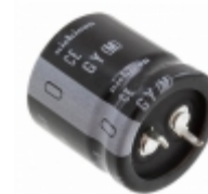
LGY1J152MELA25 Nichicon CAP ALUM 1500UF 20% 63V SNAP
