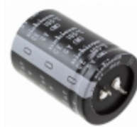
LGY1J103MELC50 Nichicon CAP ALUM 10000UF 20% 63V SNAP
