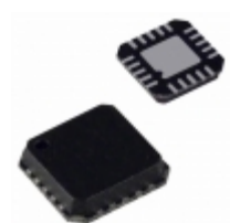
ADM8839ACPZ-REEL7 Analog Devices Inc. IC CHARGE PUMP REG TFT 20LFCSP
