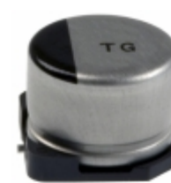
EEE-TG1E470P Panasonic Electronic Components CAP ALUM 47UF 20% 25V SMD
