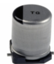
EEE-TG1E681UN Panasonic Electronic Components CAP ALUM 680UF 20% 25V SMD
