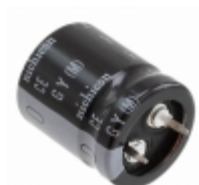
LGY1J122MELZ25 Nichicon CAP ALUM 1200UF 20% 63V SNAP
