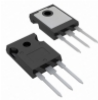
IRG7PH46UD-EP Infineon Technologies IGBT 1200V 108A COPAK247
