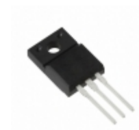
BA30BC0T Rohm Semiconductor IC REG LDO 3V 1A TO220FP
