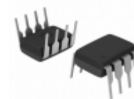
AT25640-10PI-2.7 Microchip Technology IC EEPROM 64KBIT 3MHZ 8DIP
