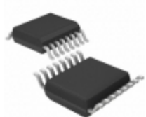
AQS221FR2S Panasonic Electric Works RELAY OPTO 40V 0.16A SOP16
