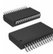
PIC24FJ256GA702T-I/SS Microchip Technology IC MCU 16-BIT 256KB FLASH 28SSOP
