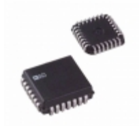
AD7537KP Analog Devices Inc. IC DAC 12BIT LC2MOS DUAL 28-PLCC
