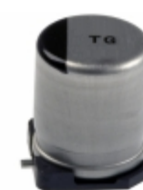
EEE-TG2A221M Panasonic Electronic Components CAP ALUM 220UF 20% 100V SMD
