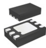
AD5611ACPZ-RL7 ADI (Analog Devices, Inc.) IC DAC 10BIT SPI 6LFCSP
