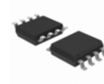
MCP4162T-104E/SN Microchip Technology IC POT DGTL SNGL 100K RHEO 8SOIC
