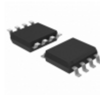
MCP4162T-502E/SN Microchip Technology IC POT DGTL SNGL 5K RHEO 8SOIC
