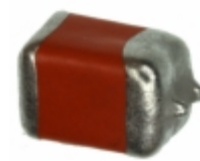
13008-040KESZ/HR Electro-Films (EFI) / Vishay CAP TANT 220UF 20V 10% 2917
