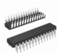
STK12C68-PF55 Cypress Semiconductor Corp IC NVSRAM 64KBIT 55NS 28DIP
