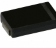
477XMPL002MG19A Illinois Capacitor CAP ALUM POLY 470UF 20% 2V SMD
