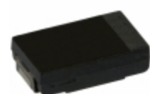
EEF-SX0D471E4 Panasonic Electronic Components CAP ALUM POLY 470UF 20% 2V SMD
