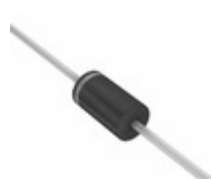
1N6289-E3/54 Vishay Semiconductor Diodes Division TVS DIODE 45.4VWM 80.5VC 1.5KE
