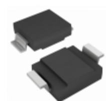
SMCG30A-E3/9AT Electro-Films (EFI) / Vishay TVS DIODE 30V 48.4V DO215AB
