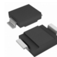
SMCG28CAHE3/9AT Vishay Semiconductor Diodes Division TVS DIODE 28VWM 45.4VC SMC
